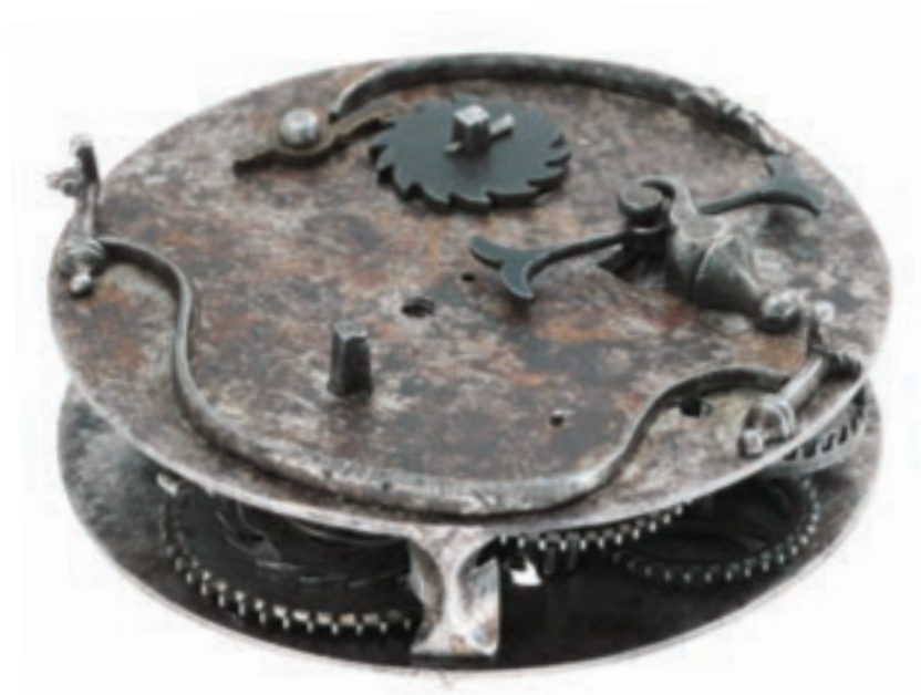
ABOVE. Movement backplate with winding square to the lower left. The foliot (which acts in the same manner as a balance) has T-shaped ends.
